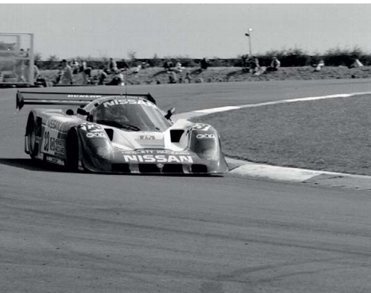
Nissan's Group C breakthrough result was a third place at Donington Park in 1989, where the R89C raced for the first time with carbon brakes and a six-speed version of the Hewland VGC gearbox
