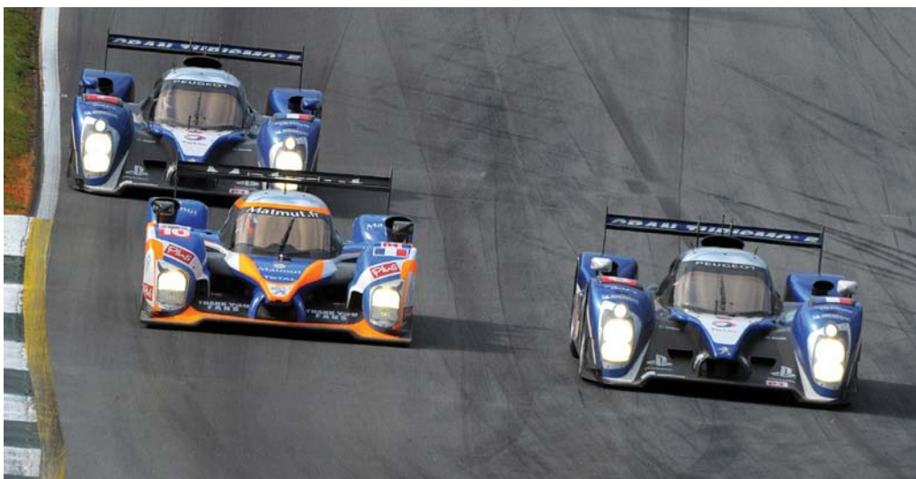
Seen here in 2009, the ORECA customer Peugeot 908 (with orange livery) features the old rear wing uprights, while the two factory cars sport the new swan neck uprights
