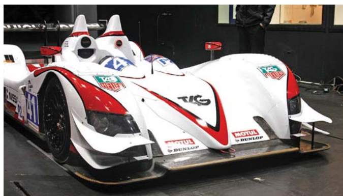
The potent front end featured the regulated splitter and double dive planes, as well as a curvaceous diffuser below
