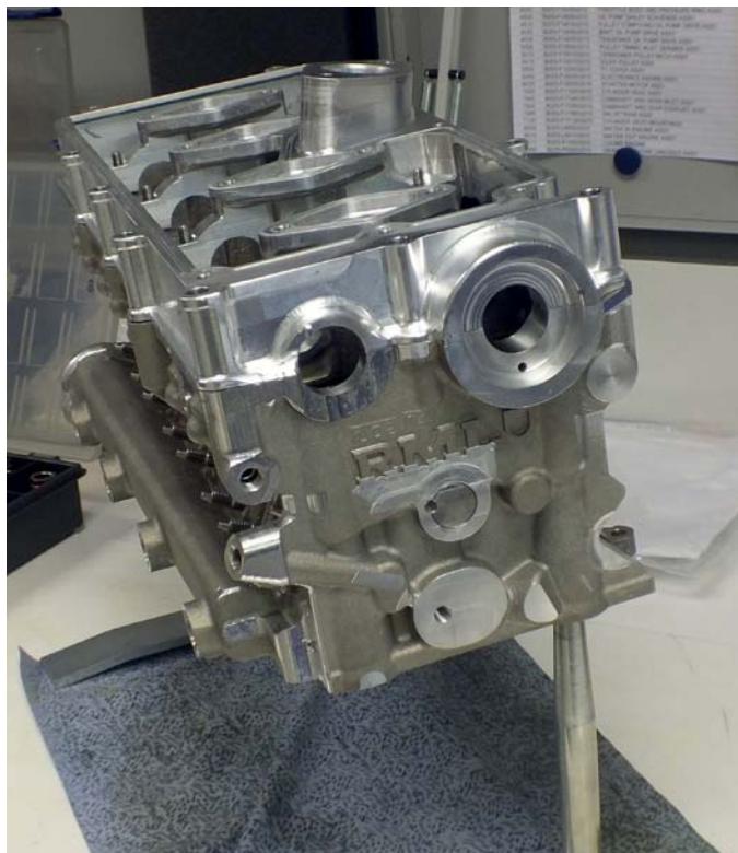
Above: every part of the engine was designed by RML, including the non-structural aluminium block, that weighs just 15kg
