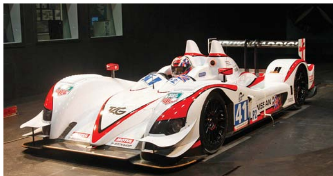
The Le Mans-winning Greaves Motorsport LMP2 Zytek Z11 SN waits for the wind in the MIRA full-scale facility
