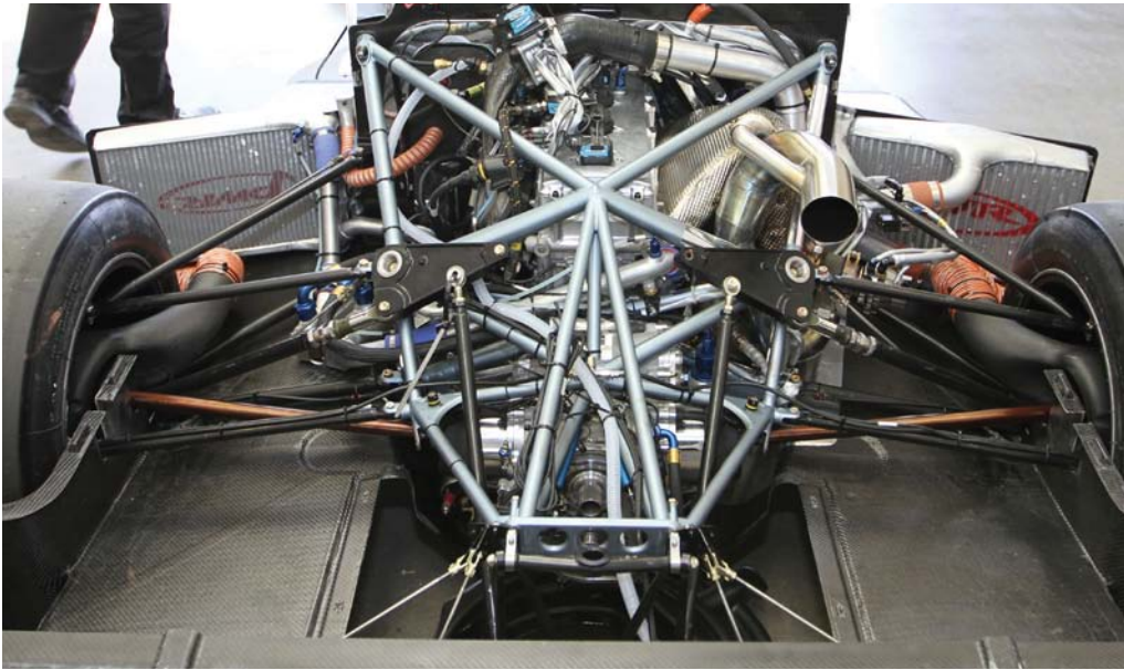
Rear suspension is a combination of conventional pull and pushrod suspension thinking, with the dampers overdriven in roll but not in heave as the roll damping of the whole car is achieved solely at the rear
