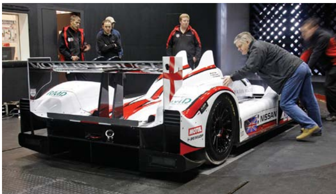
While much of the rear end is tightly regulated, the wheelarch flip ups and large rear body Gurney will be adding downforce
