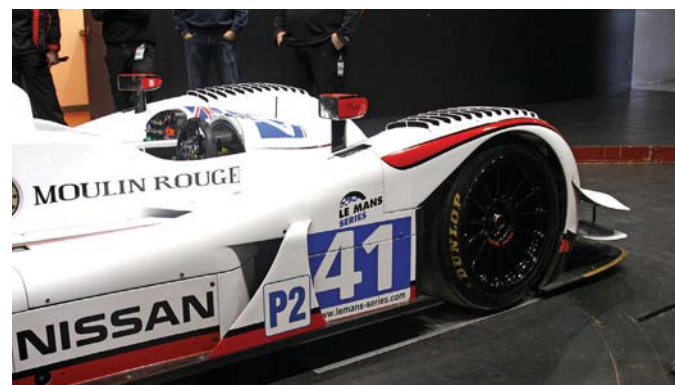
Side vents were supplemented by turning vanes
