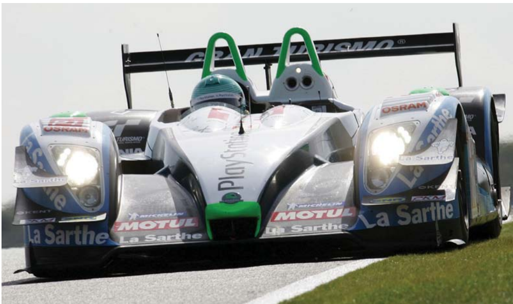
The reduction in rear wing span is immediately apparent in these pictures of the 2008 (top) and 2009 (bottom) Pescarolo. And while lap times did slow straight afterwards, other factors came into play at the same time, including the introduction of domed skids beneath the car that increased ride height and improved safety
